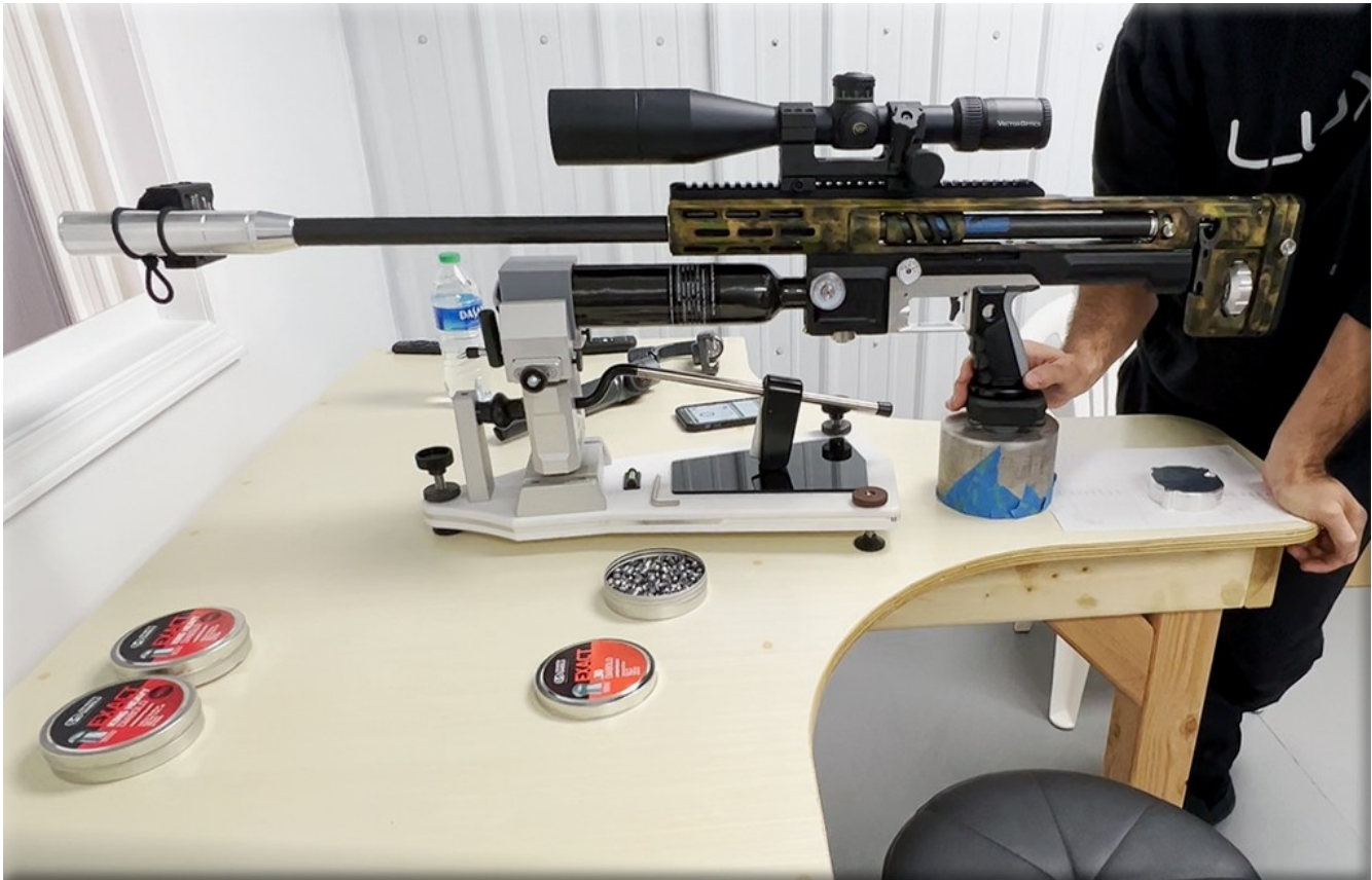
Skout Epoch Pre-production test bed model. 30 caliber; 890mm ten land 1/38 twist electronic PCP rifle.
